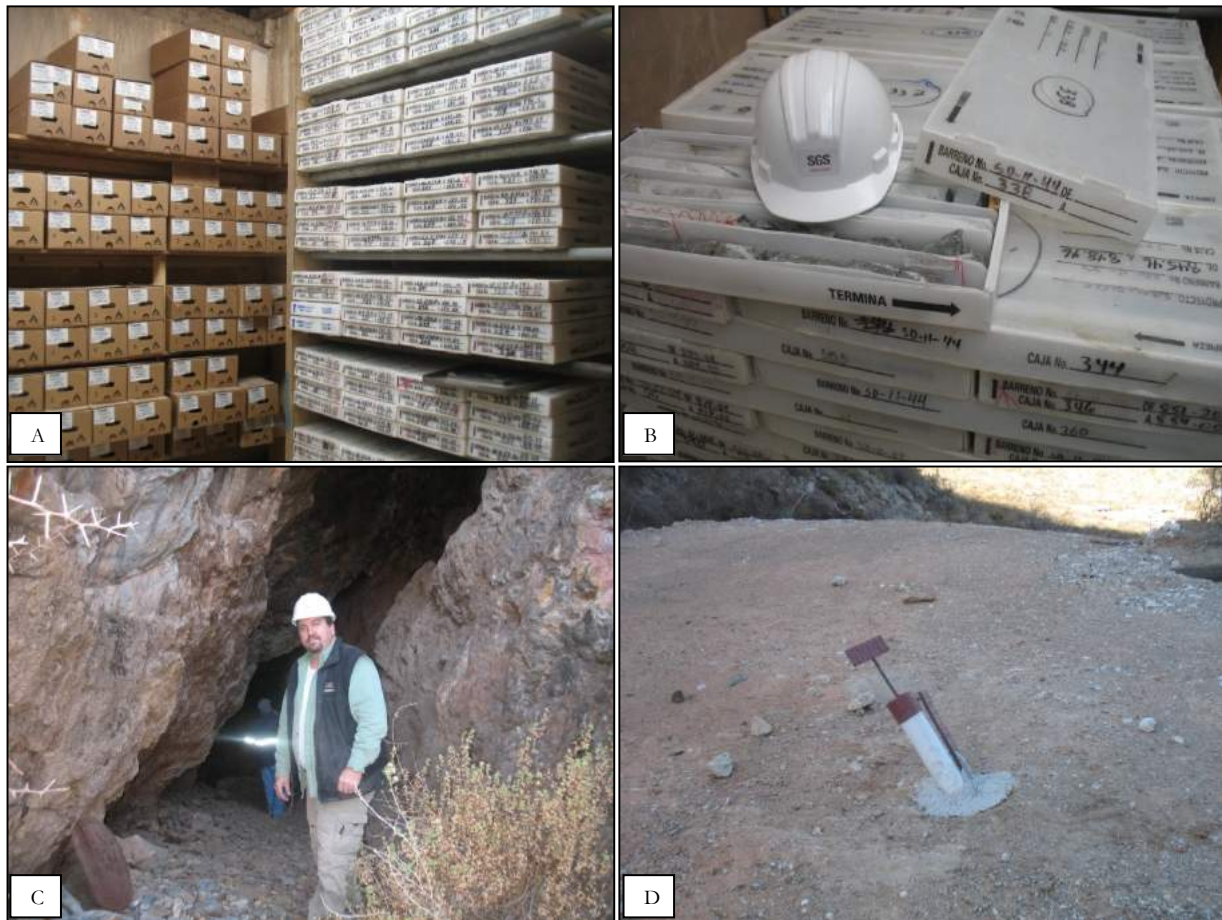
Figure 44: Photos taken by SGS consultant Claude Duplessis during the site visit. A) Core and pulp storage facility inside warehouse. B) Witness core during site visit. C) Claude Duplessis entering an old drift of the La Cruz Vein historical workings D) Drill hole SD-11-42, casing with coordinates confirmed with GPS.
