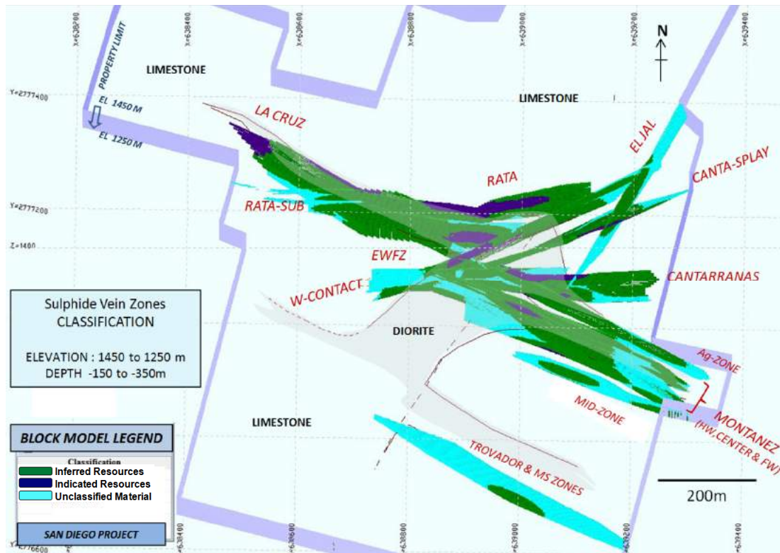
Figure 16: Plan section (-250m depth) above the Fernandez zone showing the relationship between the veins.
